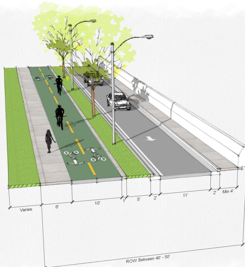
Two-Way Bicycle Facility with Planting Strip
